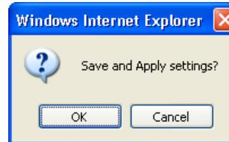
Selecting Ok to the above question will activate most Quick Config settings. Some parameters, like the IP address of the Vega, will however require the Vega to be re-booted. If a reboot is required the Vega will ask whether this should occur immediately or whether you wish to do it manually later. If later is selected, the reboot button on the left hand side menu will be left RED to indicate that a reboot is still required to activate certain new parameters.
